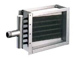
Steam coils are manufactured from thick walled copper tubes and heavy gauge copper headers with flow drilled holes for a strengthened joint.
